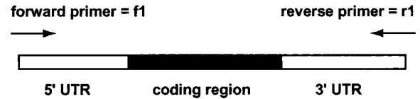
FIGURE 1.—Derivation of ESTs. Sequences generated using the forward and reverse primers correspond to the 5' and 3' ends of the cDNA clones and are denoted with f1 and r1, respectively, at the end of their sequence identification number. cDNAs were directionally cloned using asymmetric primers and linkers as described in BELL-PEDERSEN et al. (1996).
