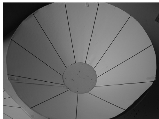
Figure 3. Funnel Cage Lined with Coated Paper Carrying Radial Lines to Provide Visual Features
