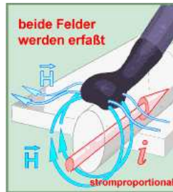
Figure 58: Langer EMV Technik RFU 5-2 near field probe
